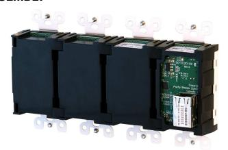
RS485 variant uses two sixpin headers (compression fit and IDC connectors) to allow multi-drop data buses. RS485 stations must be connected to a 539x NSB Architectural Gateway
